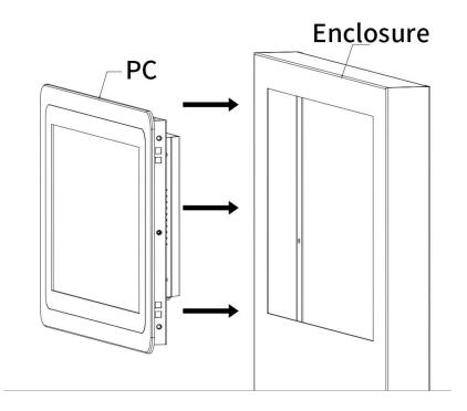
Step 2: Fix the snaps on the mouting holes of the PC, and tighten the snaps with screwdriver.
