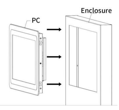
Step 2: Fix the snaps on the mouting holes of the PC, and tighten the snaps with screwdriver.
